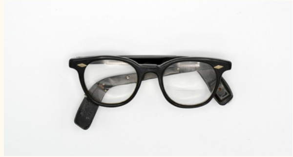
Otarion Electronics' Model Rx 880, a plastic binaural eyeglass hearing aid, 1967. This device used transistors, an electronic component invented in the mid-1900s that made the miniaturization of hearing aids possible.
